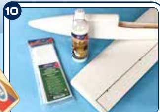
10 A second coat of Eze-Kote is applied after the glass cloth has been trimmed. After sanding and further filling if required, the model is ready for painting.
