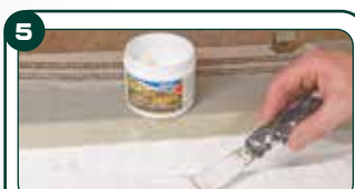
Refine the polystyrene surface using Create and Shape , and then rub flat with fine abrasive.
