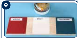
9 Here you can see we've shown Eze-Kote is compatible with Tamiya acrylic, Glass Kote epoxy and HMG cellulose paints. It will also accept conventional dope.
