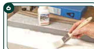
The foam surface must be sealed before painting using Foam Armour , a thick gloopy liquid.
