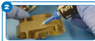
You can use Perfect Plastic Putty for scratch or dent repairs. Just squeeze a thin line of putty from the tube.
