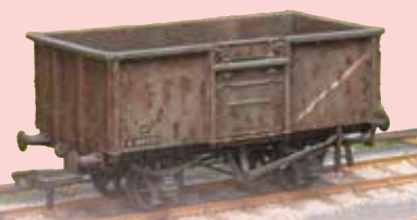
A dirty brown and dark grey weathering powder was lightly brushed over the exterior and interior using downward strokes, creating final streaking effects.
