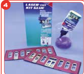
Rest the glue tip on a damp sponge to avoid it's blocking while the glue dries.
