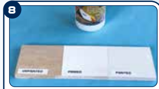
8 Having sanded the wing, we tested Halfords White primer, and our chosen paint, Halfords Spray Ford Diamond White. Eze-Kote has good compatibility with most white car primer paints. If you're in doubt always check by testing the primer and paint top coat before committing to the model.
