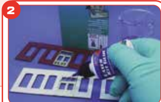
All the doors and windows were easily bonded with a thin layer of glue which easily penetrated the joint.
